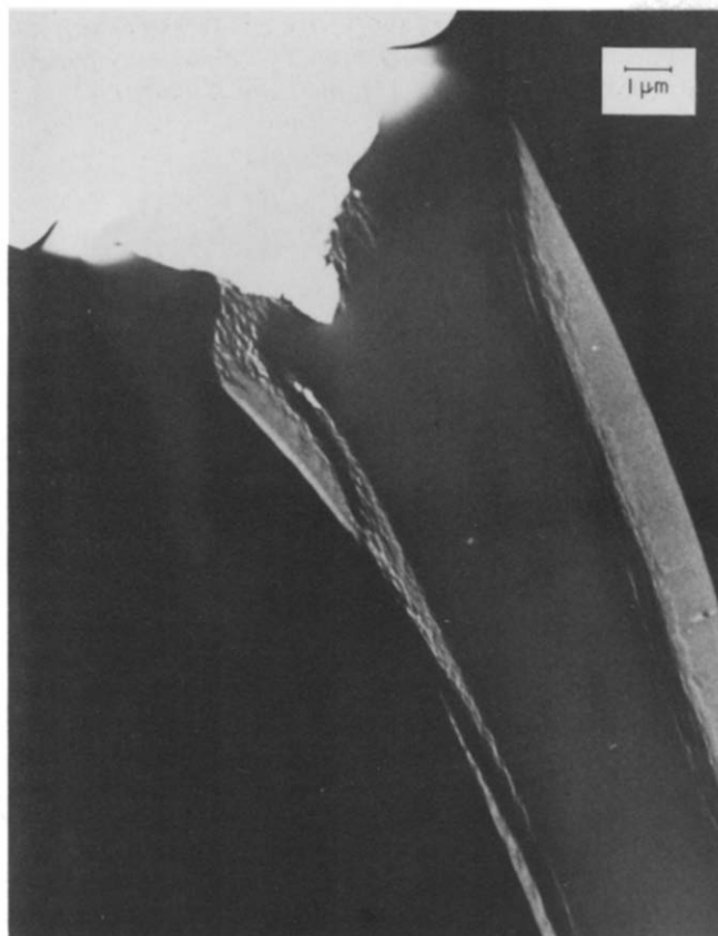
Figure 4 Growth of crazes at the edges of a zone in a PPO film which had been annealed for 2 h at 132°C
